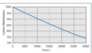
PHILIPS ESSENTIAL LEDtube has a lifetime of 25,000 hours, defined as the number of hours when 50% of a large group of identical lamps below 70% of its initial lumens.
